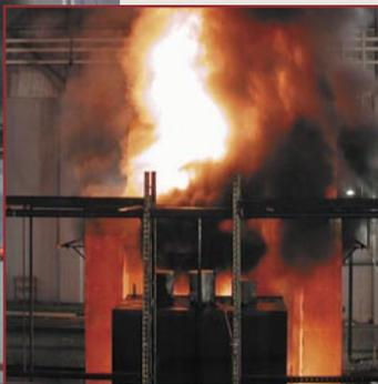
*Three types of fires—spray, pool and three-dimensional spill—are associated with turbine generator hazards.*
