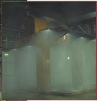
*The turbine-hall mock-up was fabricated from steel, rather than the traditional concrete, to make it more “portable.”*
