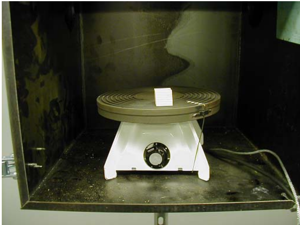
Photo of inside of smoke generation chamber
