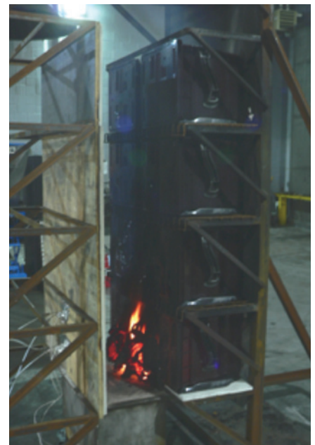
At top: A fire test of non-approved, polycarbonate containers;
