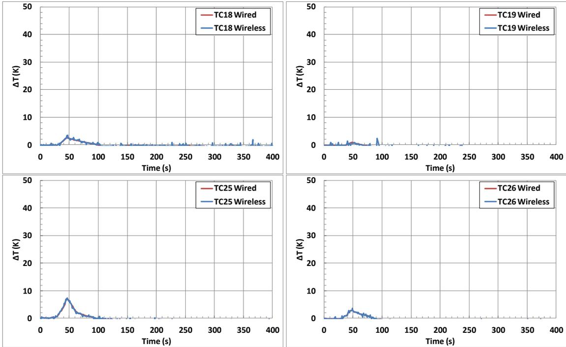
Figure A-3: Temperature rise near ignition location in Test 1.
