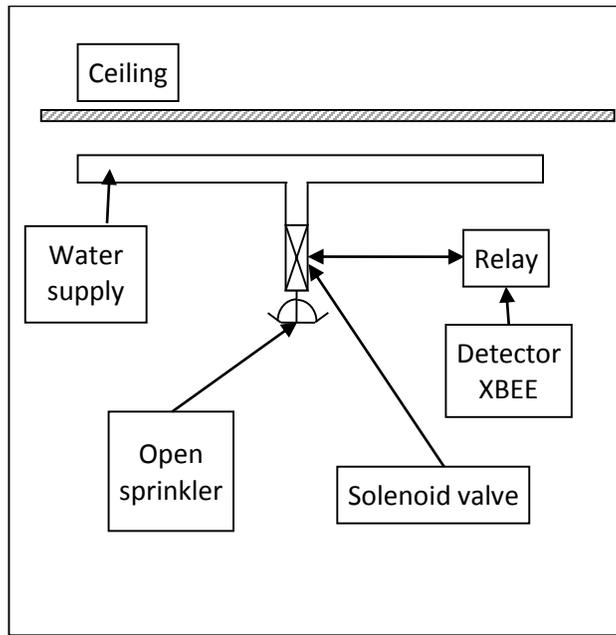
Figure 2-9: Solenoid valve and sprinkler connections.
