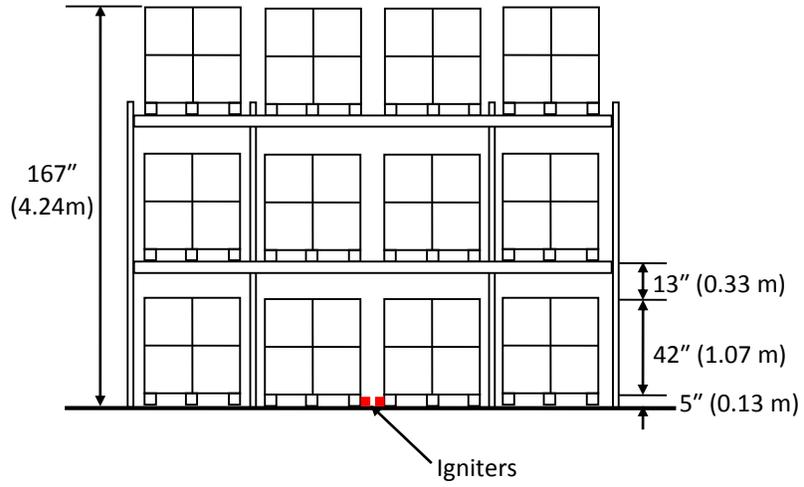
Figure 2-1: Elevation view of 2x4, 3-tier fuel array setup.
