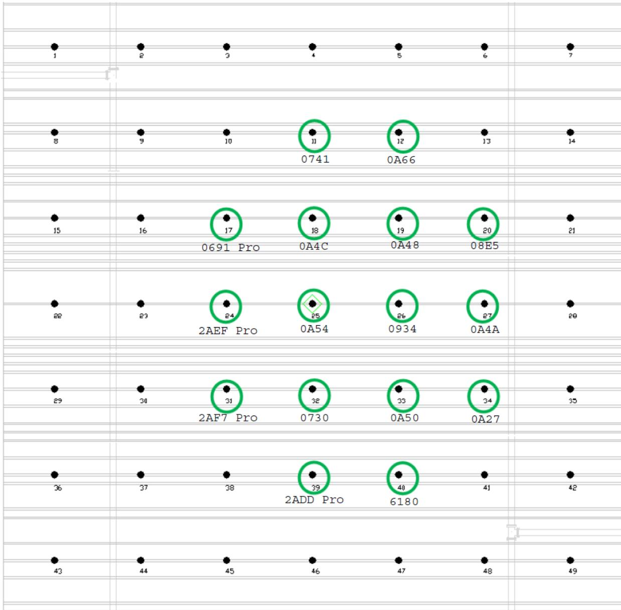
Figure 2-10: Sprinkler layout under the ceiling: 16 SMART sprinklers (green circles with ID labels below) installed on a grid with 3.05 m x 3.05 m (10 ft x 10 ft) spacing.
