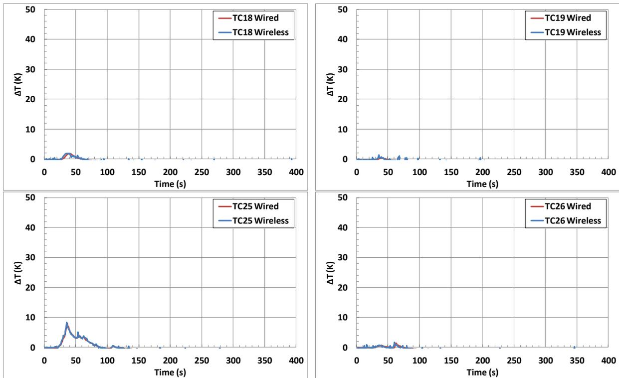
Figure A-6: Temperature rise near ignition location in Test 2.
