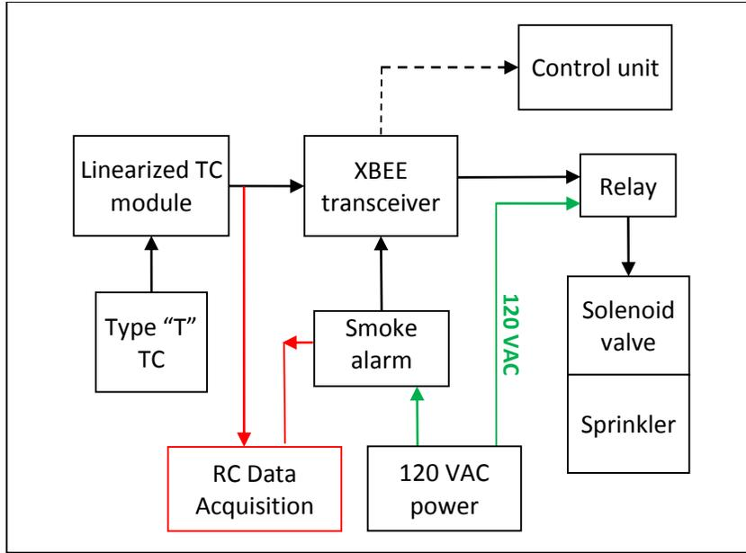
Figure 2-8: Smart sprinkler node connection.
