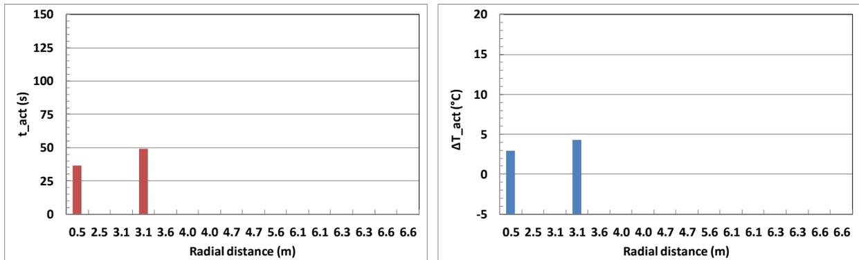
Figure A-2: Smoke alarm activation times and temperature rise in Test 1.
