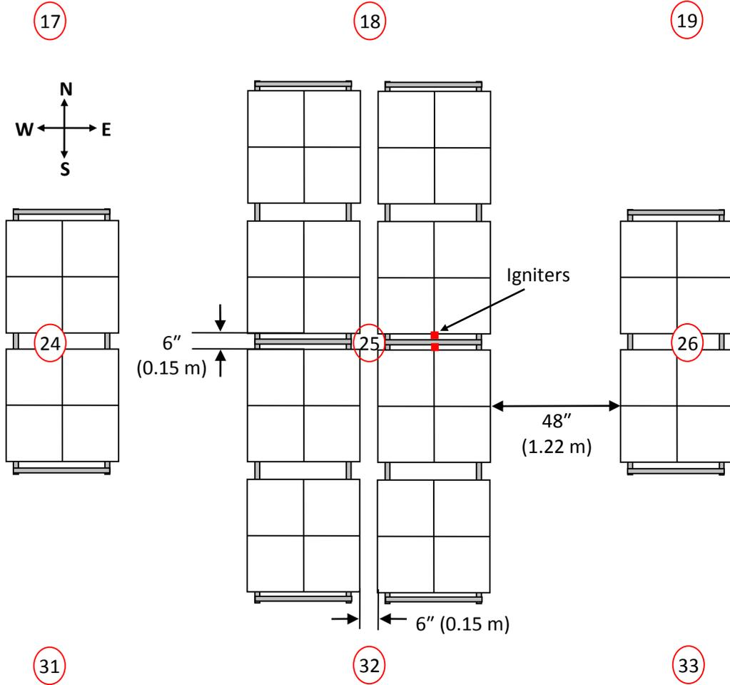
Figure 2-6: Plan view of sprinkler layout and fuel array: Test 1-2, Under 1 Offset.
