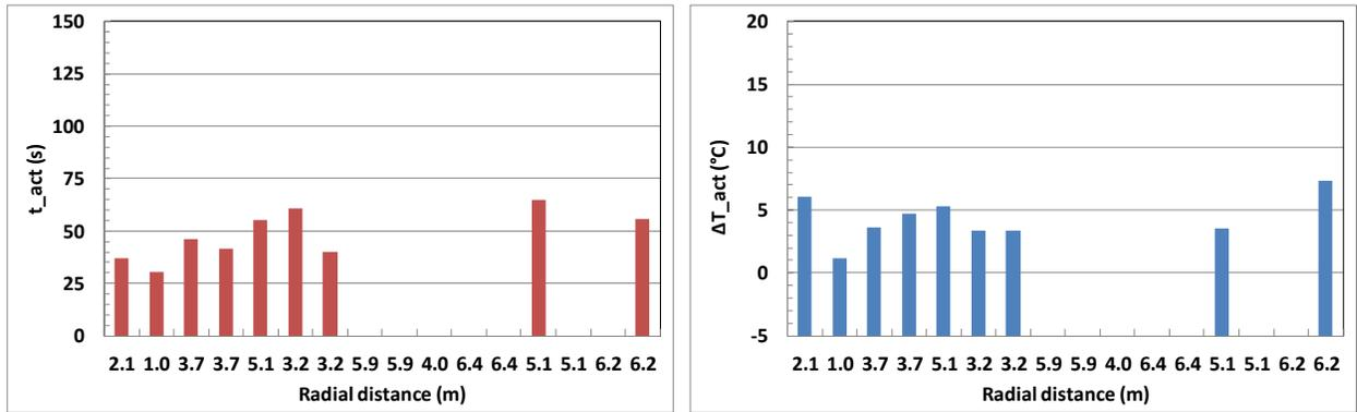
Figure A-8: Smoke alarm activation times and temperature rise in Test 3.
