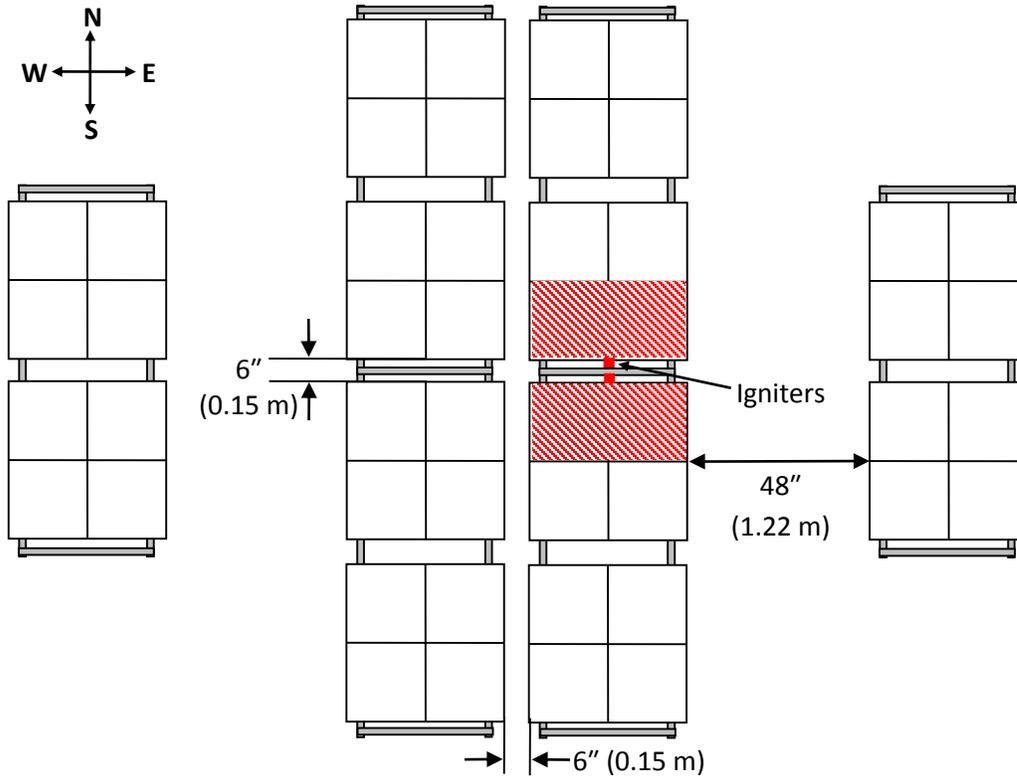
Figure 3-13: Plan view of fire damage (red hachures) at the bottom tier in Test 3.
