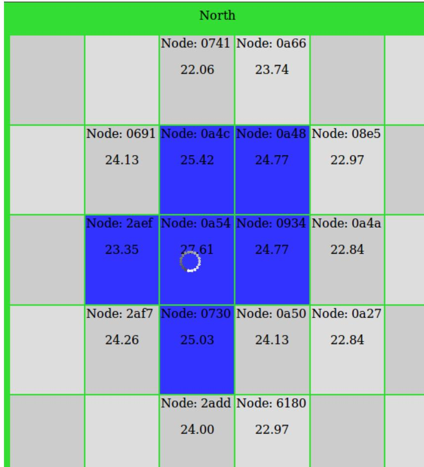
Figure 3-2: Sprinkler activation with under-1 ignition in Test 1.
