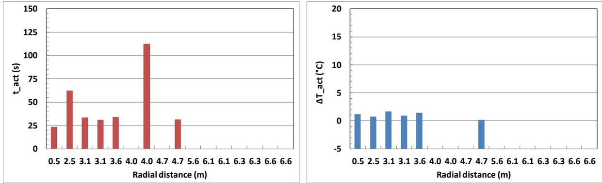
Figure A-5: Smoke alarm activation times and temperature rise in Test 2.
