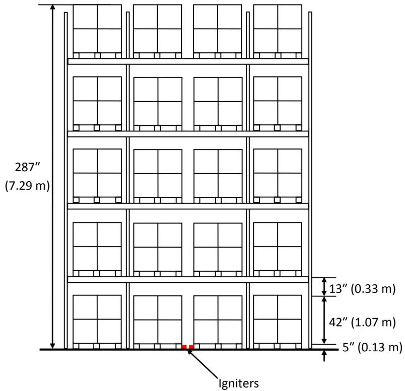
Figure 2-2: Elevation view of 2x4, 5-tier fuel array setup.
