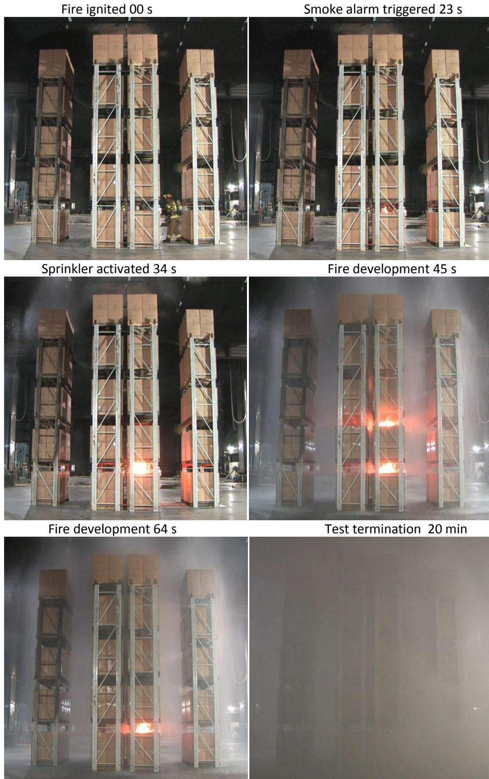
Figure 3-8: Fire development in Test 2 [K200, 26.5 mm/min (K14.0, 0.65 gpm/ft<sup>2</sup>)].
