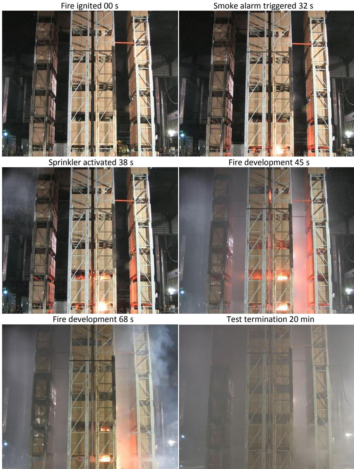
Figure 3-12: Fire development in Test 3 [K360, 36.6 mm/min (K25.2, 0.9 gpm/ft<sup>2</sup>)].
