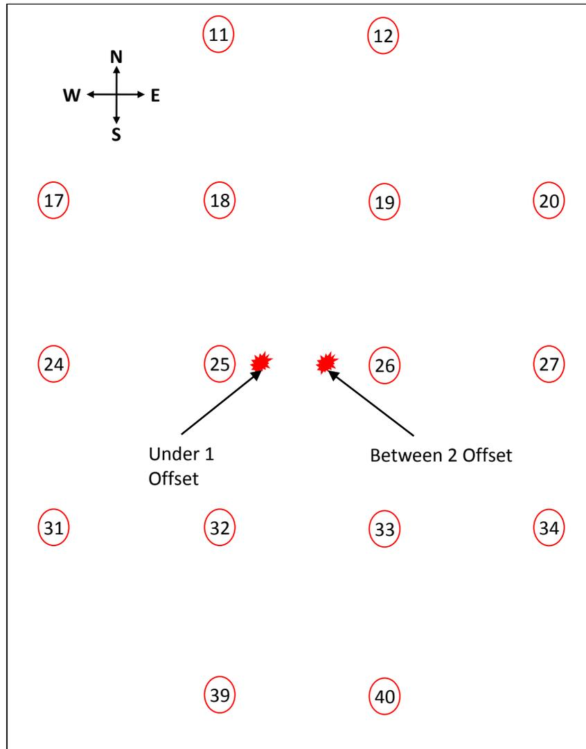
Figure 2-5: Smart sprinkler layout under the south movable ceiling with 3.05 m × 3.05 m (10 ft × 10 ft) spacing.
