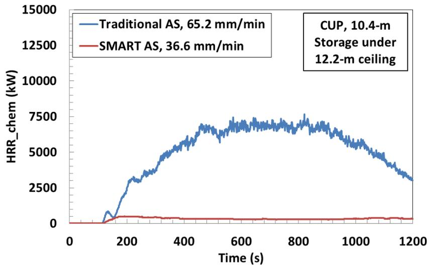
Figure 3-14: HRRs in 7-tier CUP rack storage tests using traditional and SMART sprinklers.
