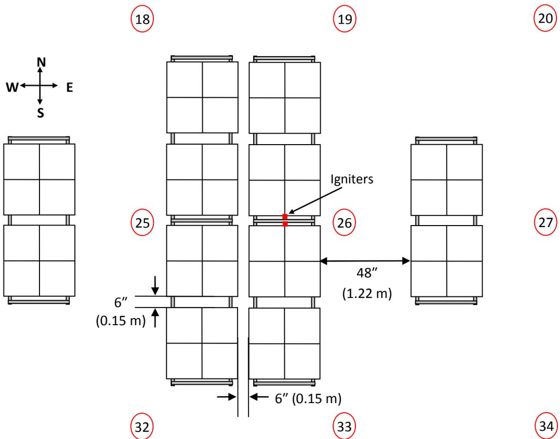
Figure 2-7: Plan view of sprinkler layout and fuel arrays: Test 3, Between 2 Offset.
