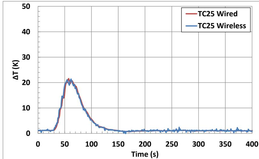
Figure 3-10: Temperature rise near ignition location (Sprinkler #25) in Test 3.
