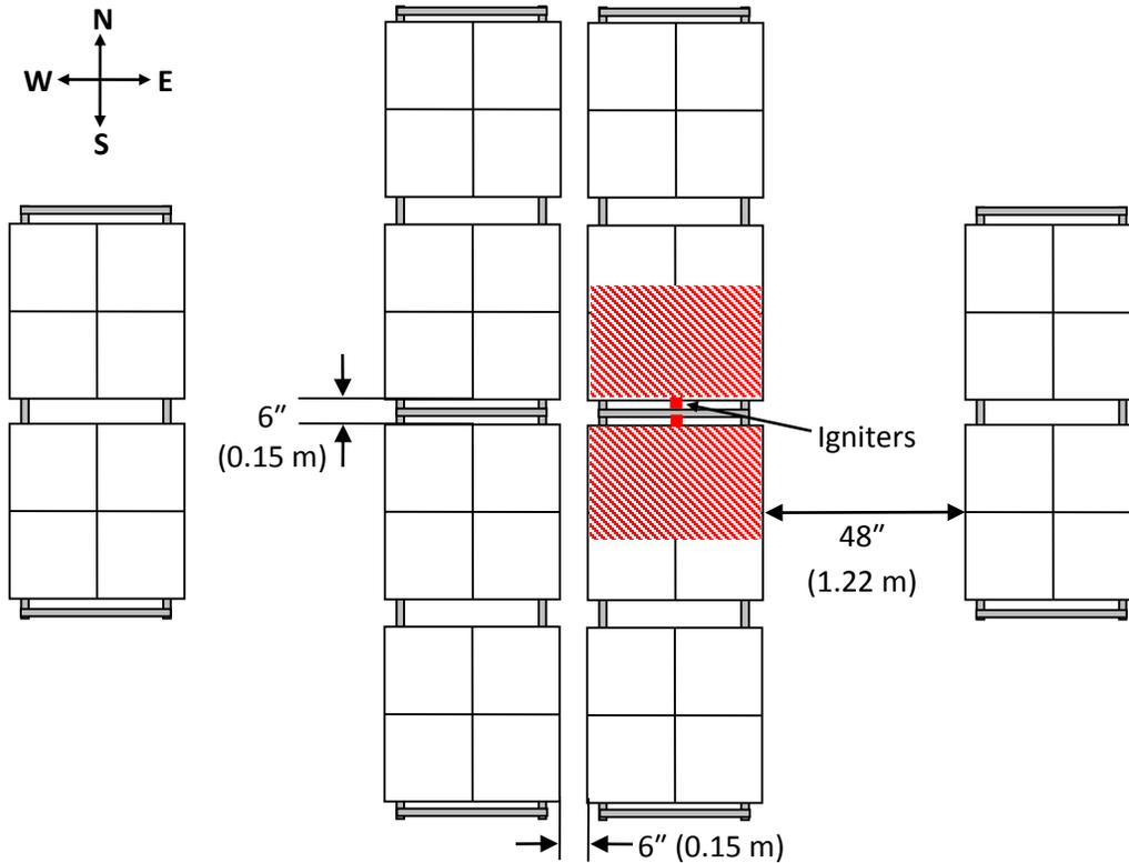
Figure 3-4: Plan view of fire damage (red hachures) limited to the bottom tier in Test 1.
