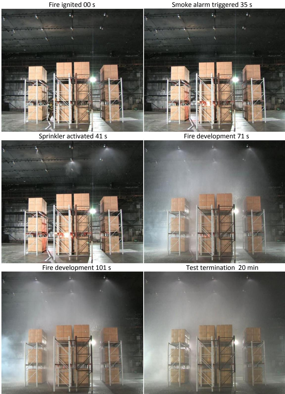
Figure 3-3: Fire development in Test 1 [K160, 16.3 mm/min (K11.2, 0.4 gpm/ft<sup>2</sup>)].
