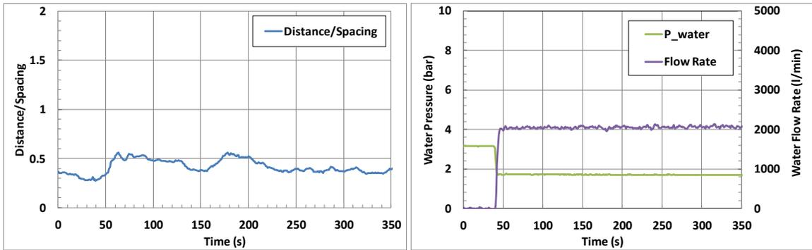
Figure A-7: Calculated thermal centroids and water discharge rate in Test 3.
