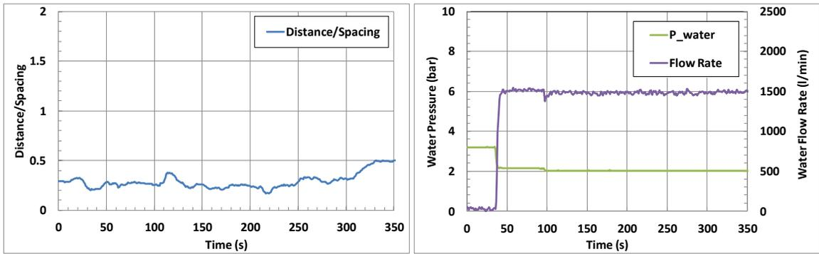
Figure A-4: Calculated thermal centroids and water discharge rate in Test 2.
