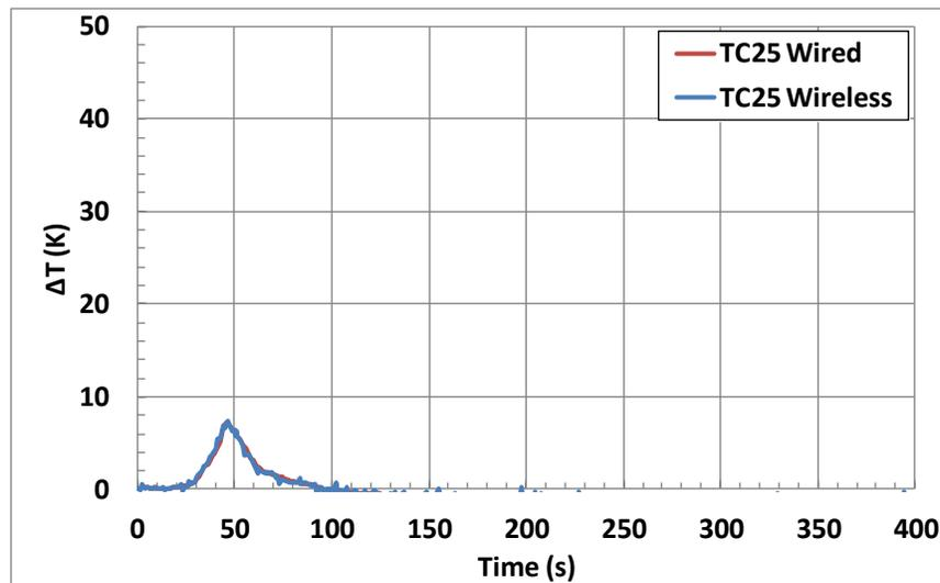
Figure 3-1: Temperature rise near ignition location (Sprinkler # 25) in Test 1.
