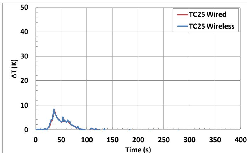
Figure 3-6: Temperature rise near ignition location (Sprinkler # 25) in Test 2.
