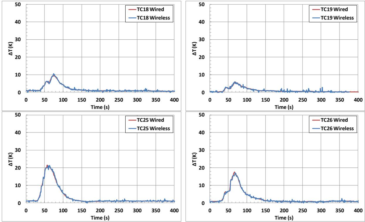
Figure A-9: Temperature rise near ignition location in Test 3.
