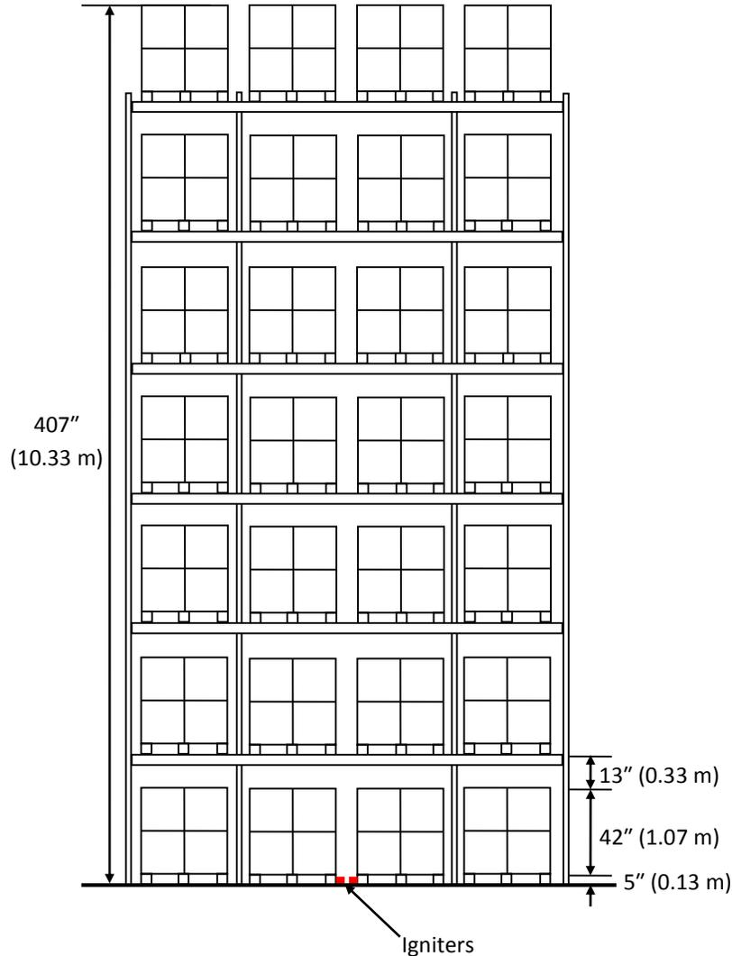
Figure 2-3: Elevation view of 2x4, 7-tier fuel array setup.
