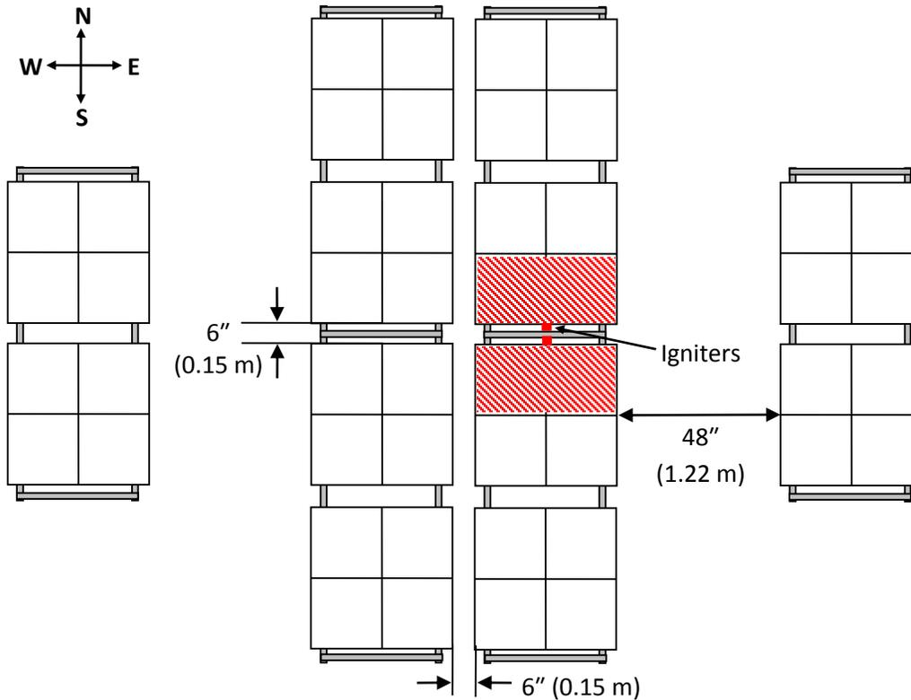
Figure 3-9: Plan view of fire damage (red hachures) limited to the 1<sup>st</sup> and 2<sup>nd</sup> tiers in Test 2.
