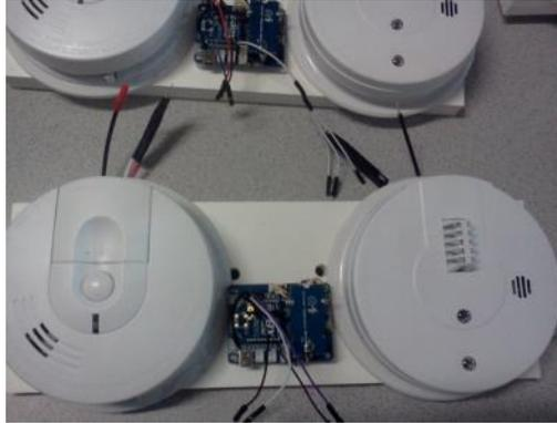
Figure 2-4: Wireless transceiver connected to smoke and heat detectors.
