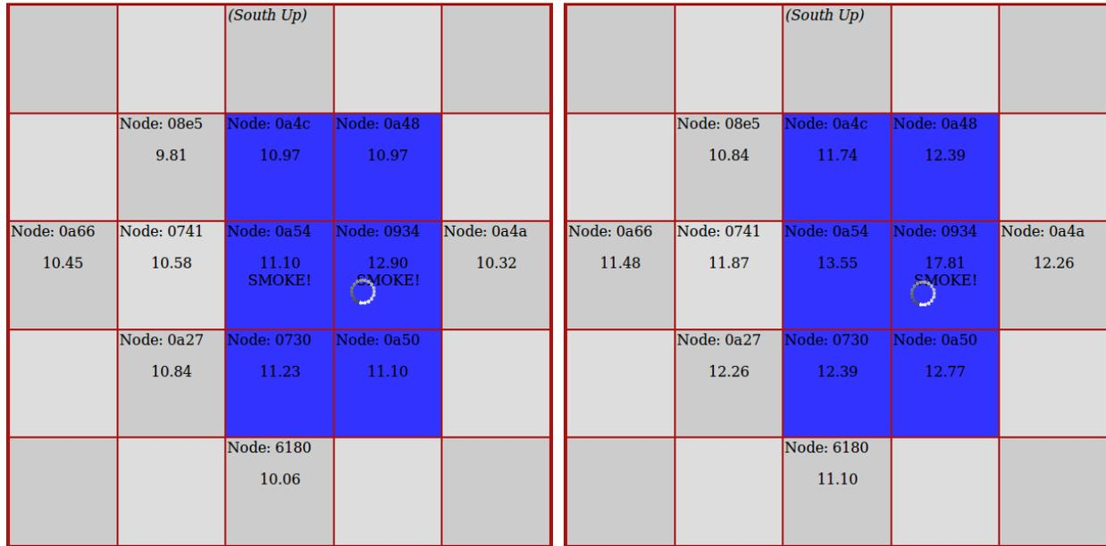
Figure 4-25: Sprinkler activation with under 4 ignition in Test 43 (L) and 46 (R).
