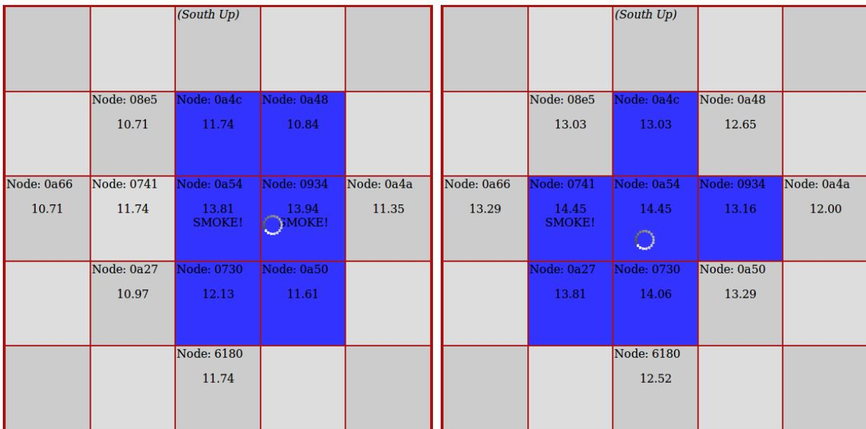
Figure 4-24: Sprinkler activation with between 2 ignition in Test 42 (L) and 45 (R).
