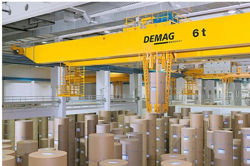
Figure 1-1: Roll paper in high on-end storage configurations (photo courtesy of Terex MHPS Corp).
