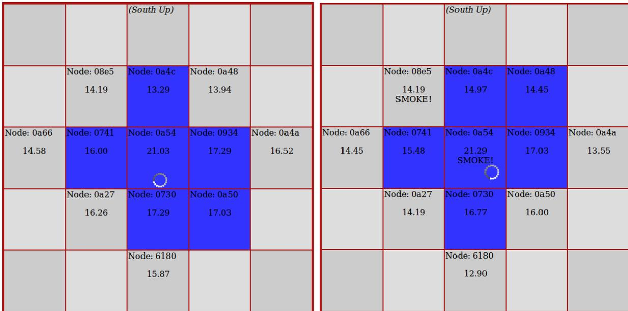
Figure 4-23: Sprinkler activation with under 1 ignition in Test 41 (L) and 44 (R).
