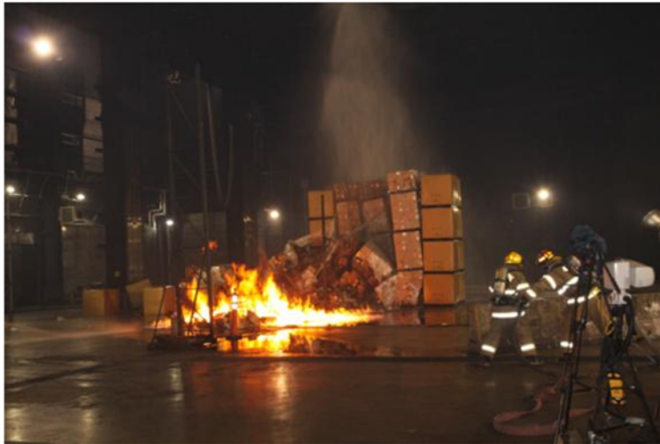
Figure 3-146: Array Collapse (20 min 36 s)
