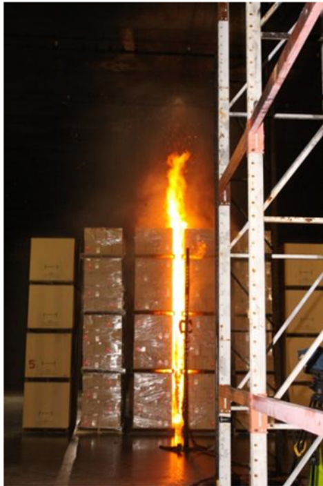
Figure 3-148: Test 2 - 1st Sprinkler Operation (1 min 12 s)
