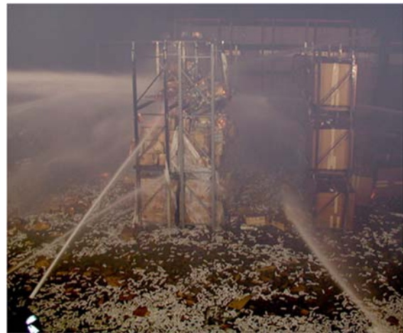
Extinguishment Efforts at About 45 minutes. Note Residual Flaming and Many Bottles in Debris.
