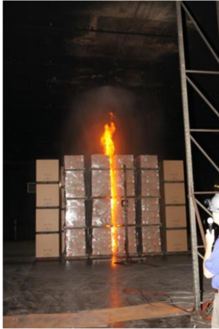
1st Sprinkler Operation (1 min 4 s)
