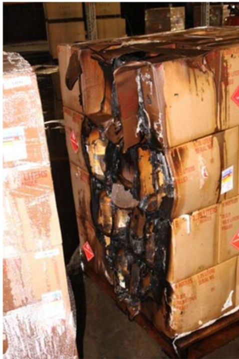
Figure 3-155: Post Test Damage to Commodity near Ignition Flue – Test 4
