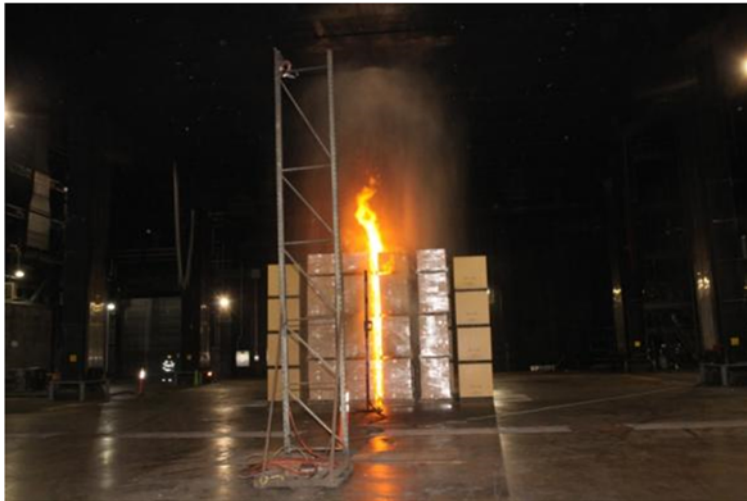
Figure 3-144: 1st Sprinkler Operation (1 min 19 s)
