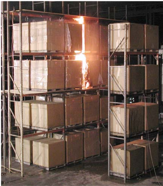
Fire Development at 1:57 Two Seconds Prior to Initial In-rack Sprinkler Operation.
