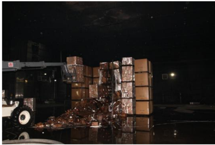
Figure 3-152: Test 3 - Array Collapse During Cleanup (Post Test)
