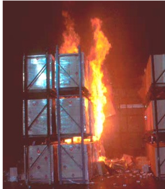
Fire Progress at 1:27, Eight Sprinklers Operating; Flames Steady on ceiling.
