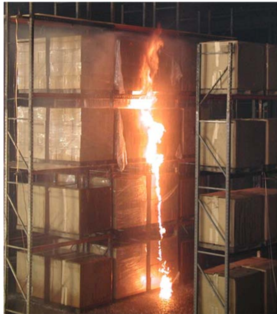
Fire Progress at 4:19, Final Total of Three In-rack Sprinklers Operating.
