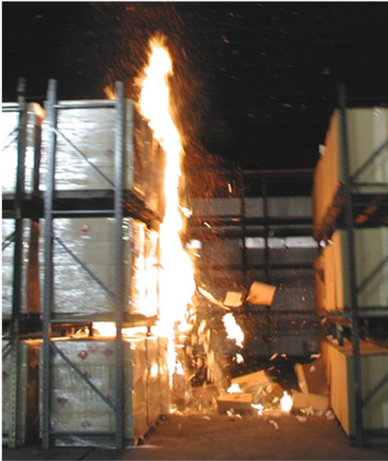
Major Explosion at 0:55; Flames on Ceiling (9.1 m [30 ft] High).
