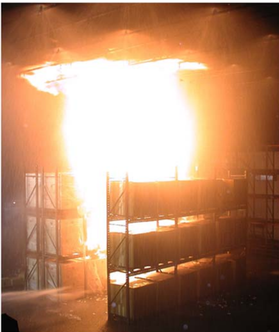
Fire Progress at 1:54 When Test Was Terminated. 33 Operating Sprinklers; Six Seconds Later 54 Sprinklers Were Open.
