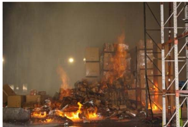
Collapsed Material (5 min 50 s)
